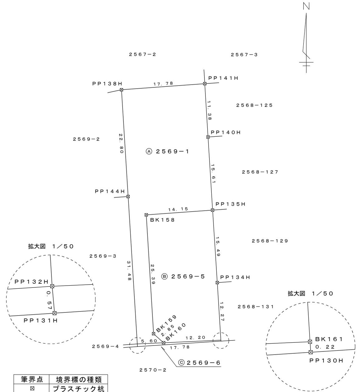
Table with 2 columns: 筆界点 (Boundary Point) and 境界標の種類 (Boundary Marker Type). Shows plastic stakes (プラスチック杭).
